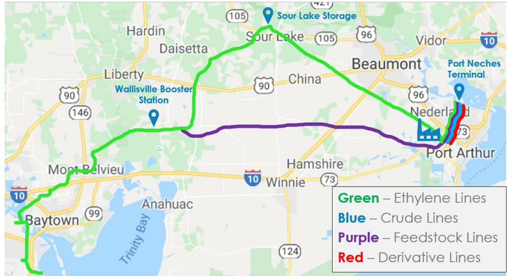
Petroleum and petrochemical pipeline infrastructure includes pumping stations that are used to manage pipeline flow and pressure, interconnection stations that allow for product to flow from one pipeline system into another, and breakout tankage that provides temporary storage along the pipeline system.
